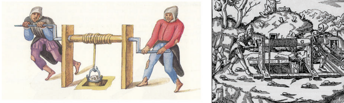
Figure 2. Picture of a winch in (left) the Schwazer Bergbuch (Innsbruck, Tiroler Landesmuseum, Codex Dip. 856, f. 123) and (right) Agricola's De re metallica (Basel 1556, p. 118).
